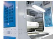
The machine includes: stainless steel vibrating tiers for pasta surface drying; a drive system with metallic elastic bars; adjustable product advancing speed; outer panels made of insulation material covered with stainless steel; high-efficiency heating batteries equipped with a temperature control probe; a humid air extraction unit consisting of internal pipes, a centrifugal electrofan and a regulating valve.
