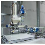
Vacuum tight flour doser. Single-shaft, high-speed pre-mixer. Stainless steel mixing tank equipped with a probe for dough level control. The whole mixing process takes place under vacuum. In the mixer a slow rotating shaft enables the achievement of the optimal hydration time, besides enhanc-
