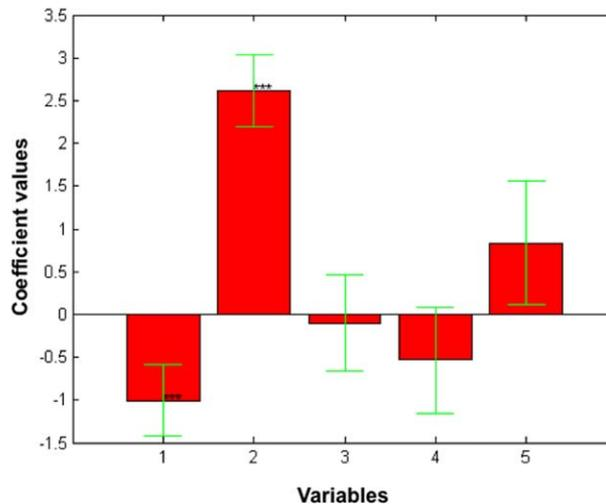
**FIGURE 5** Coefficients plot of the variables for the MLR model on  $M_e$ . 1. Temperature, 2. Relative humidity, 3. Nut dimension, 4. Shell thickness, 5. Empty space. \*\*\*( $p < .001$ ) \*\*( $p < .01$ ) \*( $p < .05$ )
