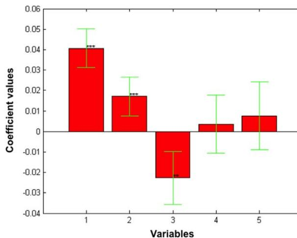
**FIGURE 6** Coefficients plot of the variables for the MLR model on  $k$ . 1. Temperature, 2. Relative humidity, 3. Nut dimension, 4. Shell thickness, 5. Empty space. \*\*\*( $p < .001$ ) \*\*( $p < .01$ ) \*( $p < .05$ ).
