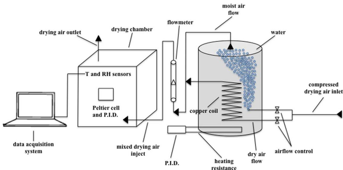
FIGURE 1 Scheme of the lab-scale drying system adopted for the experiments
