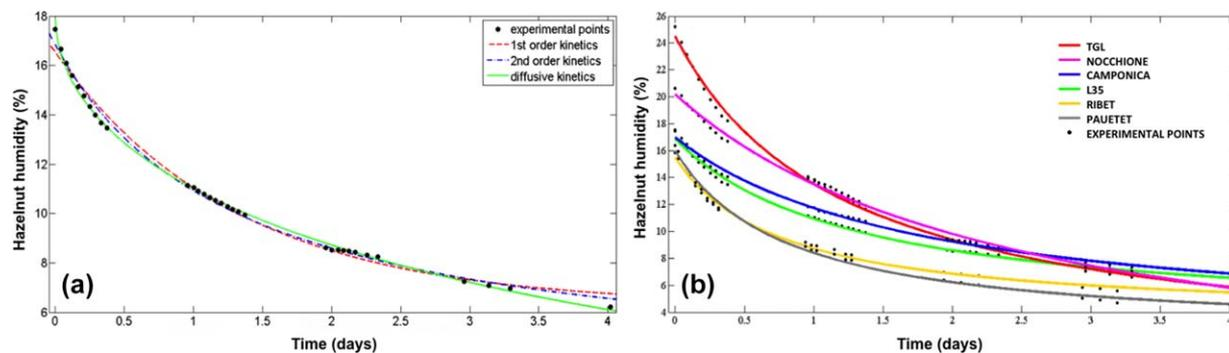
**FIGURE 2** Drying curves. (a) Comparison among fitting curves corresponding to the 1st order kinetics (dash line), the 2nd order kinetics (dash-dot line) and the diffusion kinetics based on the Fick's 2nd law (solid line) for the same cultivar [L35;  $T$  20 °C; RH 20%]; (b) Comparison among the changes of moisture content during drying of hazelnuts belonging to the six hazelnut cultivars at the same experimental condition [ $T$  20 °C; RH 20%]
