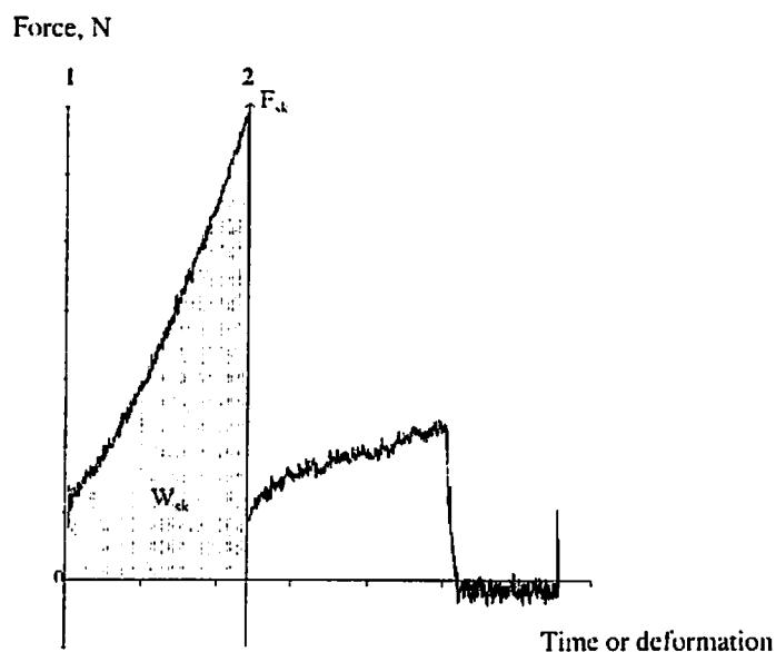
**Figure 1 – Force-time Curve corresponding to the berry skin penetration test.**
