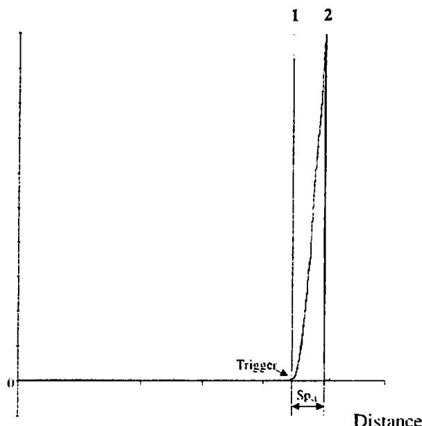
**Figure 2 – Force-distance curve corresponding to the berry skin thickness determination test.**
