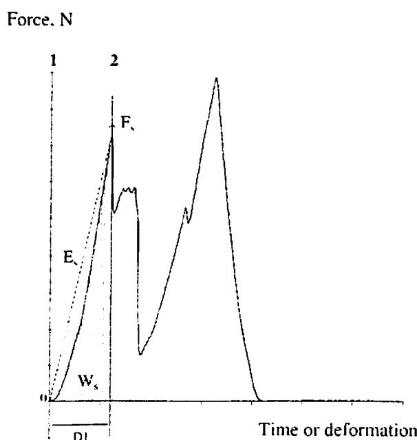
**Figure 3 – Force-distance curve related to the test for seed hardness determination.**
