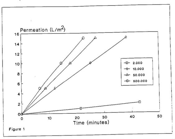
Polisulphone microporous membranes with cut-off variables from 2000 to 500000 Daltons were used for the tests. They were carried out with musts at 22 °C, average transmembrane pressure was 1.2 bar and velocity of the fluid was 3.0 m/s.
